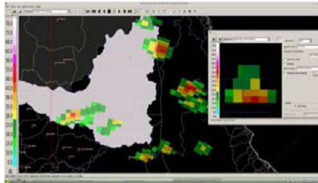
Radars monitor the growth of seeded, non-seeded cloud; monitor the development of clouds into seedable clouds; locate seedable clouds for pilot's information where to seed
