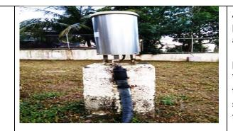
An instrument that measures precipitation and is usually attached to an event recorder. It is an upright cylinder that has a funnel-shaped receiver. The precipitation collected by the receiver empties into one side of a "tipping bucket" once filled (0.5 mm).
