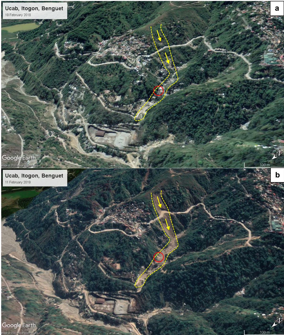
Fig. 5.2. Google Earth images of Sitio First Gate, Barangay Ucab, Itogon, Benguet on (a) 19 February 2018 and (b) 11 February 2019. The debris flow is outlined in yellow while the arrows show the direction of the landslide. The approximate location of the concrete bunker that was used as evacuation shelter by the miners and their families is encircled in red. In Fig. 5.2b, the Baguio-Bua-Itogon road had already been cleared of obstruction because the image was taken nearly 5 months after the incident.
